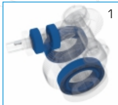
ZZ shielded pre lubricated bearings on input and output shaft
